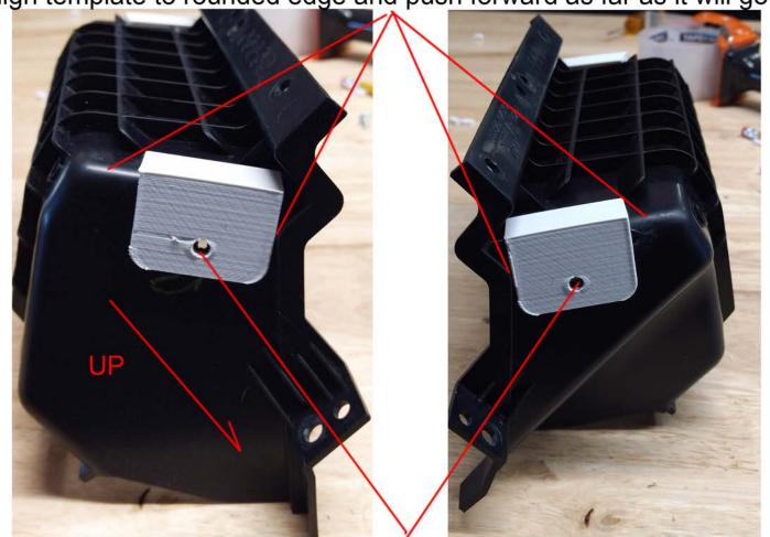
Drill 5/32 hole through template both sides
