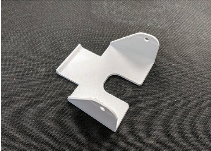
STECH-4 T4R template to drill two holes that hold in housing
