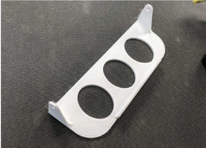
STECH-6 T4R template to drill two holes that hold in housing
