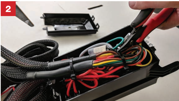
2 Remove bottom cover and cut the cable ties that hold things together.
