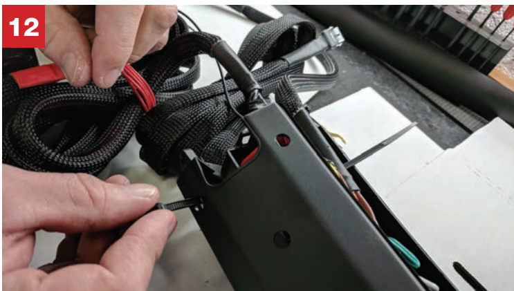
12 Reattach bottom of box while feeding a cable tie through, underneath all exiting wires from the harness, as shown.
