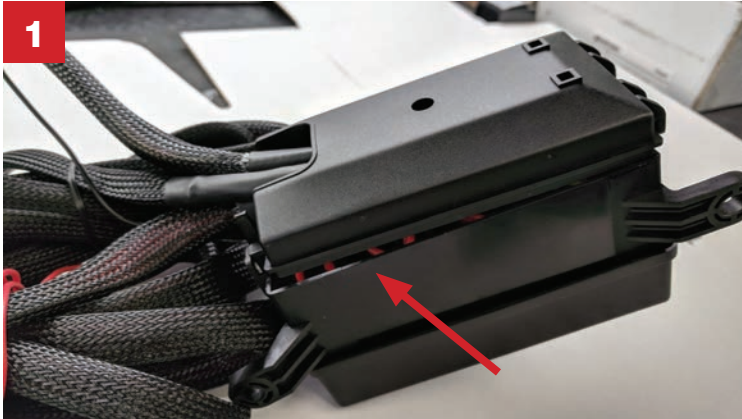
1 Showing the unwanted gap.
