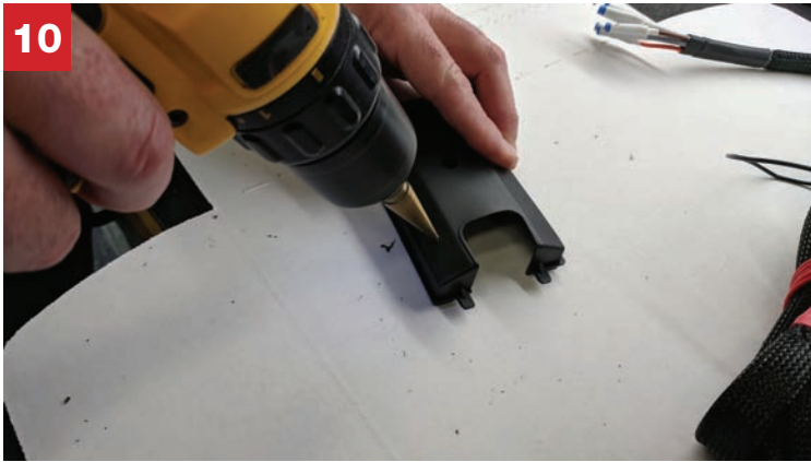
10 Drill two 1/4" holes on each side of the bottom of the box in this location - see below as well.
