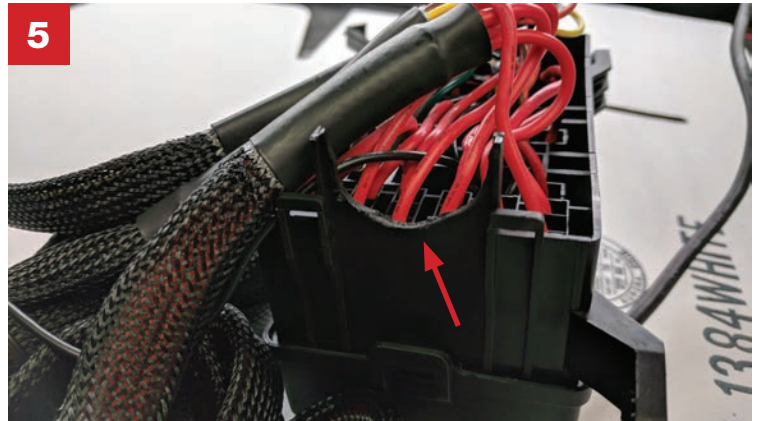
5 Showing the exit tunnel made deeper.
