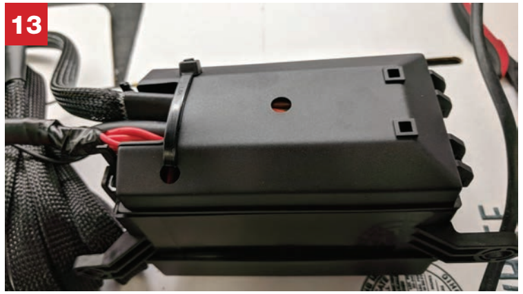
13 Secure cable tie in place.
