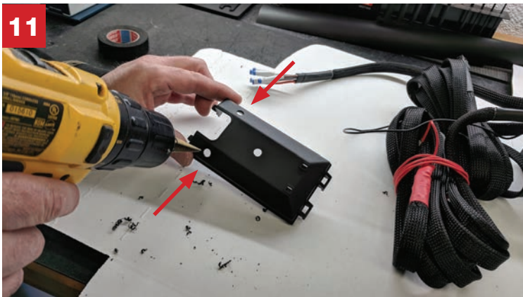
11 Showing the location of the holes to be drilled.
